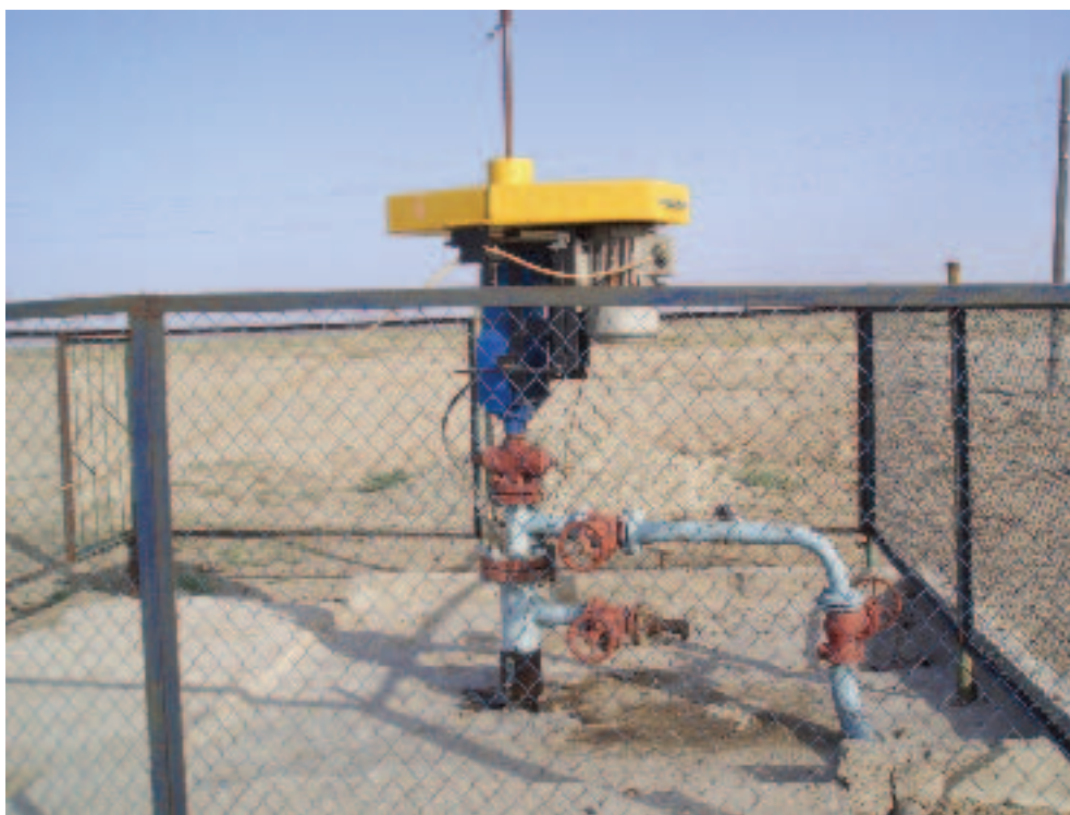
ZhaikMunaiGas NGDU Gran Field Screw Pump Oil Well
